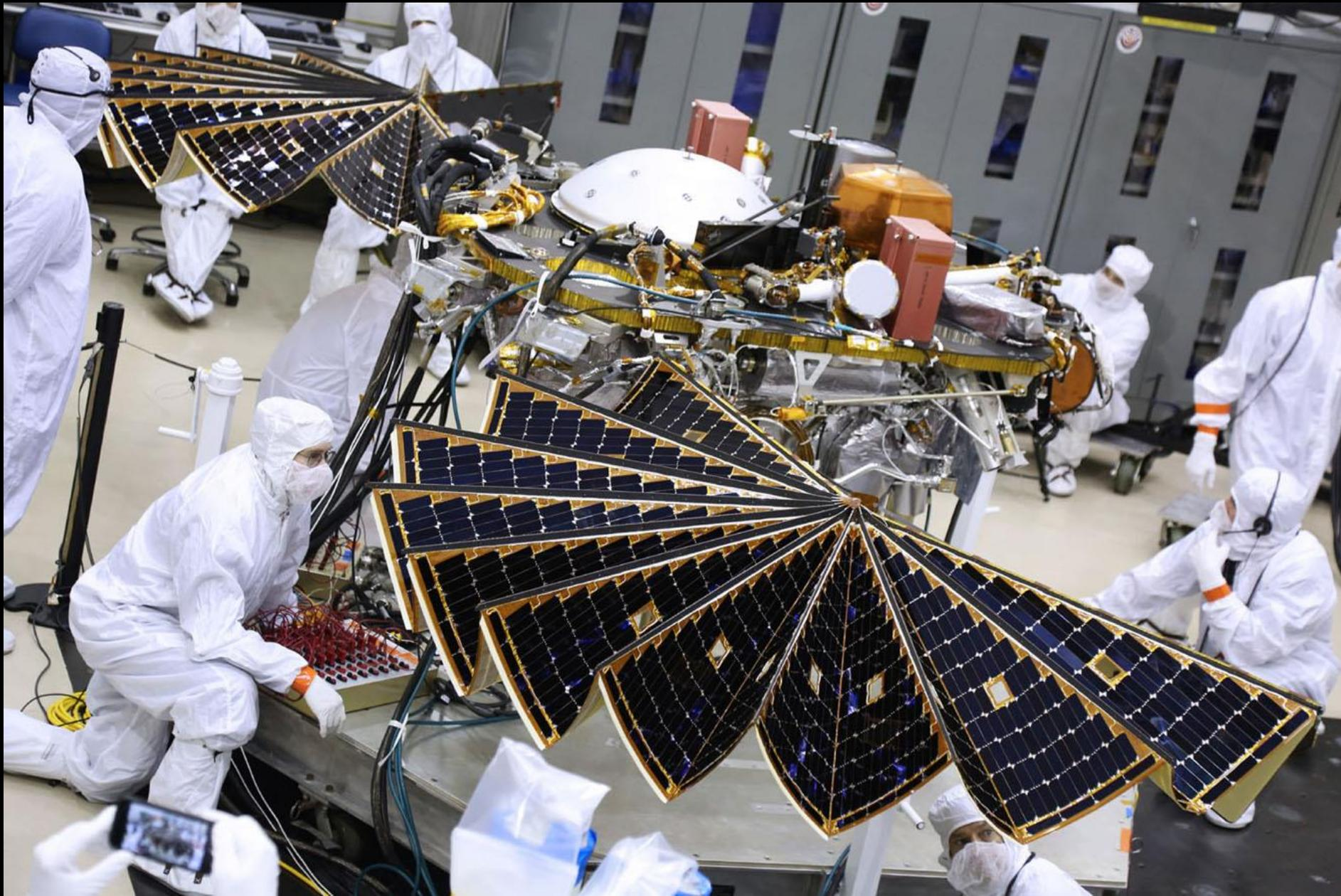
The solar arrays on NASA's InSight Mars lander were deployed as part of testing conducted Jan. 23<sup>rd</sup>, 2018, at Lockheed Martin Space in Littleton, Colorado. Engineers and technicians evaluated the solar arrays and performed an illumination test to confirm that the solar cells were collecting power. The launch window for InSight opens May 5, 2018.
