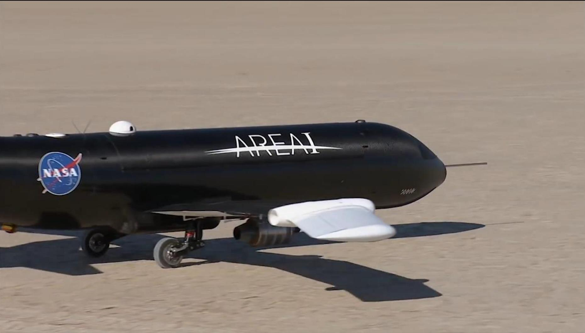
NASA has successfully applied a new technology in flight that allows aircraft to fold their wings to different angles while in the air. The recent flight series, which took place at NASA's Armstrong Flight Research Center in California, was part of the Spanwise Adaptive Wing project, or SAW. This project aims to validate the use of a cutting-edge, lightweight material to be able to fold the outer portions of aircraft wings and their control surfaces to optimal angles in flight.
